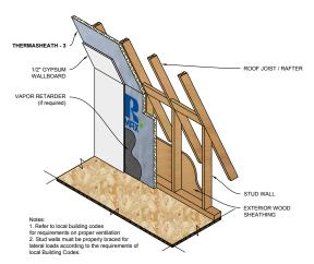
**Attics and Crawl Spaces** - Thermasheath-3 may be applied to the interior face of stud walls or roof rafters within attics and crawl spaces to provide a layer of continuous insulation (ci). Simply nail the Thermasheath-3 to the framing members and cover with an approved ignition barrier such as 3/8" gypsum wallboard or 1/4" wood structural panel, particle board or hardboard.
